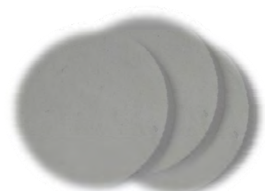
Cast foam A Specimens M11, M12, M13 Thickness: 19.68 mm Diameters: 44.44 mm
