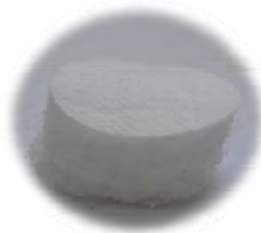
Non homogeneous thickness (usual for limp fibrous)
