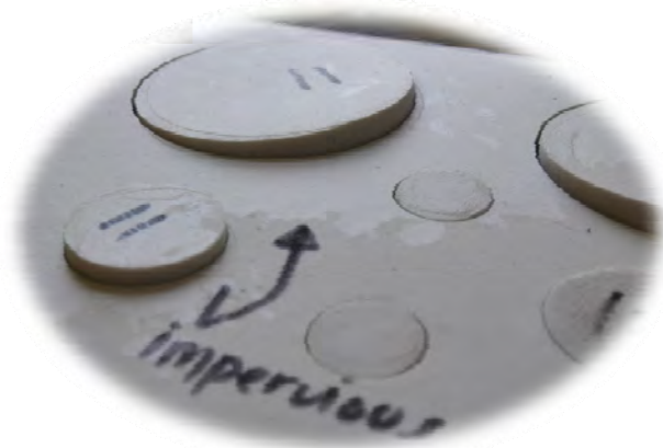
Surface defect – impervious film (usual for cast foams)
