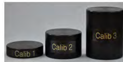
Calibration gauges (10, 25, and 50 mm thick) (for static calibration)
