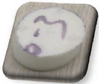
Perforated screen ( h=0.47 mm \sigma=137700 Nsm -4 ; \phi=0.08 )
